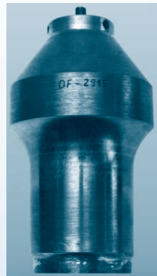
Ultrasonic welding sonotrode
