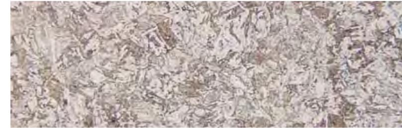
5 % Ni and 3 % Cu. Since components of this grade also have to comply with the NACE specification, only the condition DH 1150 is allowed (approved). In addition to an excellent combination of strength and toughness, the pitting resistance of these steels is also good.
